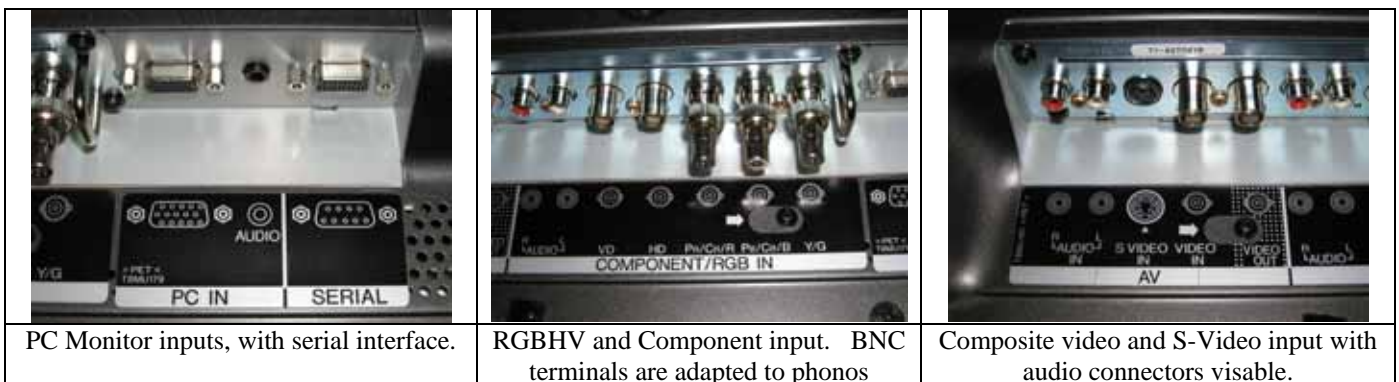
Figure 1. Available connections on the typical plasma screen. Most have the VGA monitor input with the optional terminal board to provide additional video inputs.
